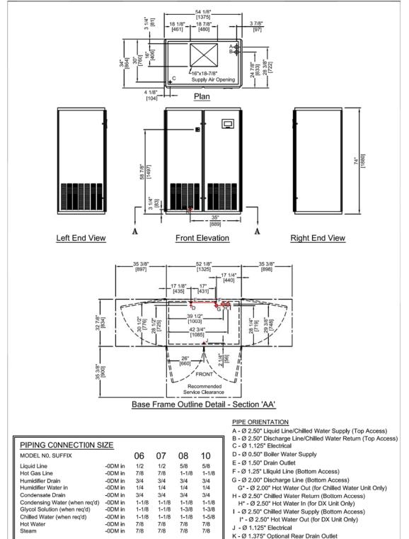
0DM - Outside Diameter of copper pipe in inches for soldering
